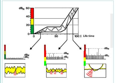
As defects in the Rolling Element Bearing develop, the amplitude of shock pulses increases. Value exceeding the dBi characterizes the damage and is used to assess the condition of the Rolling Element Bearing:
