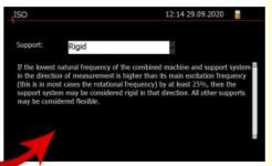
According to ISO Standard, based on machine parameters the DC-23 sets up the masurements and the alarm levels for the machine condition zones.
