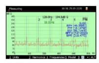
Detailed analysis of any spectrum with defect frequencies, harmonics and sidebands for modulation processes.
