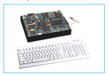
8085 Microprocessor Kit with Accessories/Peripherals and Interfacing Devices.
