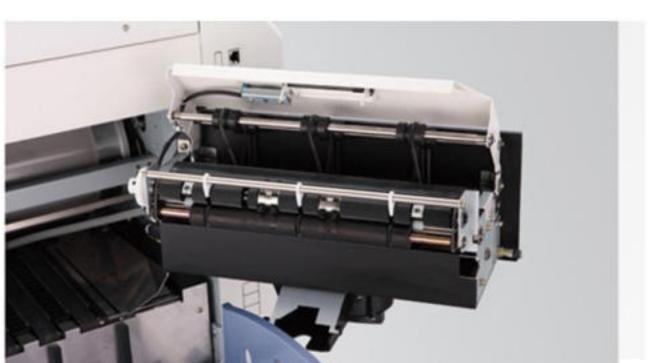
Innovative design of paper feeding by double rollers which is much more stable. Simultaneously feed paper to guarantee one page input only once.
