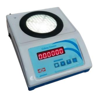
Microprocessor Based Digital Colony Counter is a suitable instrument for counting Bacterial colonies. Our diverse range of Microprocessor Colony Counter offered by us is of premium quality and is fabricated using quality raw material. With the assistance of our designers and experts we are capable to offer customized solutions to our clients as per their specifications in stipulated time frame
