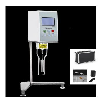
Digital viscometers operate on the principle of how a fluid's internal friction affects its flow behavior. They typically measure the time it takes for a given amount of fluid to flow through a specific geometry (usually a capillary tube or rotating spindle) under controlled conditions. The measurement is then used to calculate the fluid's viscosity
